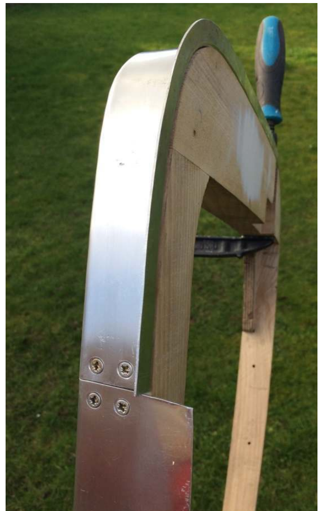
The 2 halves of the door edge meet at a butt joint.
