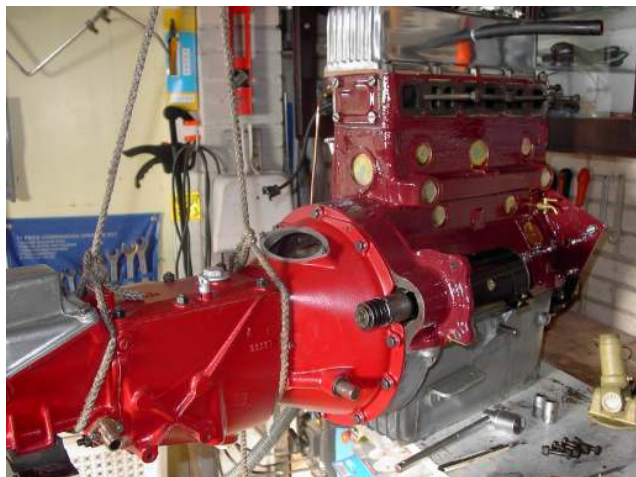
The engine and gearbox ready for installation – note new core plugs!
