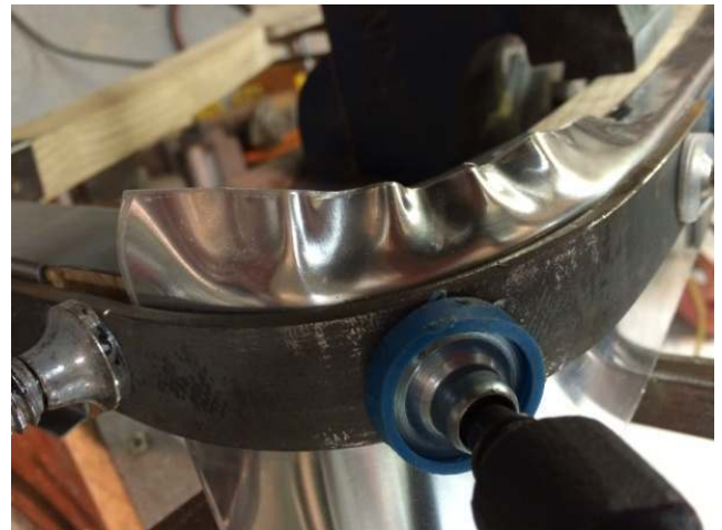
With care and cutting back to 10mm it does shrink down flat.
