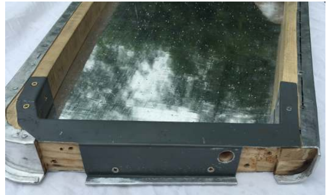
Hinge reinforcement panel with welded in corners for additional strength.
