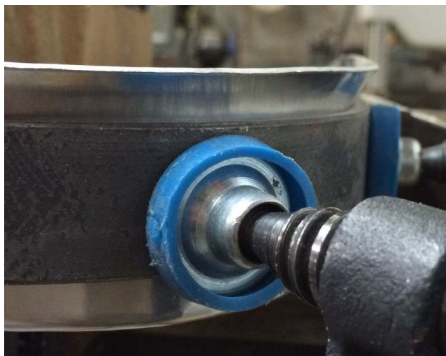
How it starts to move in a tight even curve, very different to the loose folds formed by shrinking.
