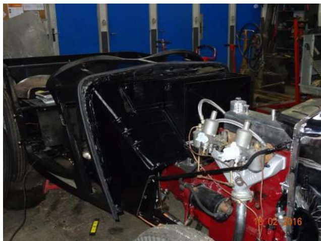
Shiny black bulkhead in place. All main bolts are in but no nuts on yet.
