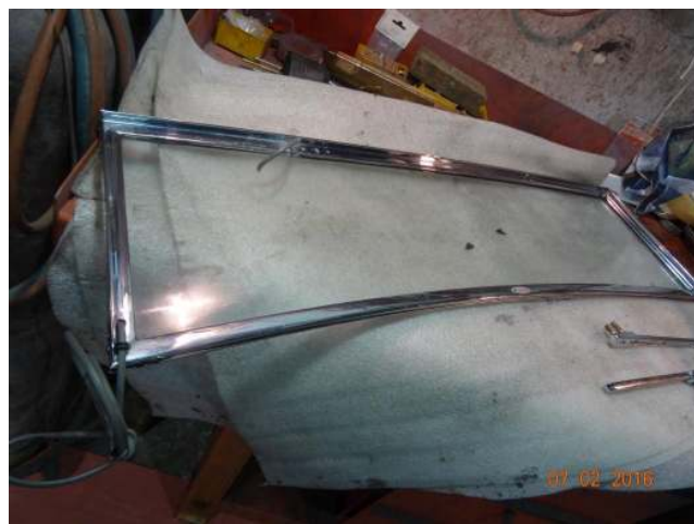
Glass now fitted to the windscreen frame.
