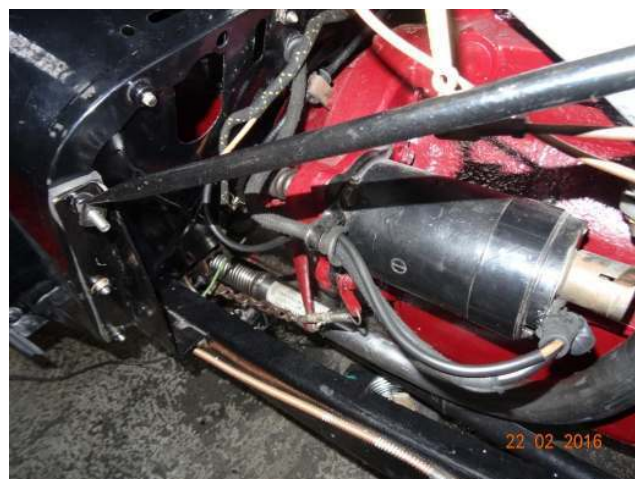
The first wire of the loom to be fitted, the brown main feed. Just visible are the two green wires hanging down by the brake switch.
