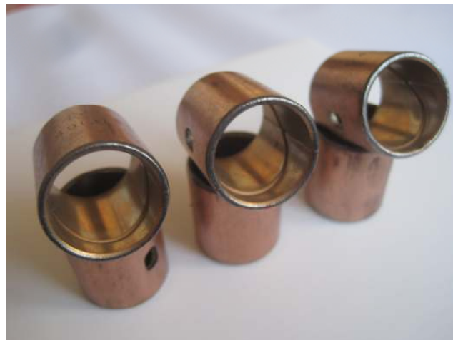
Bi-metal 'wrapped' king pin bushes – note the oil/grease groove which has a spur take off that feeds lubrication to the thrust faces of the beam axle's eye.
