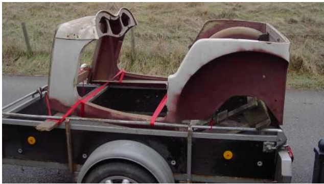
The Belgian body tub – sound panelling but shame about the timber!
