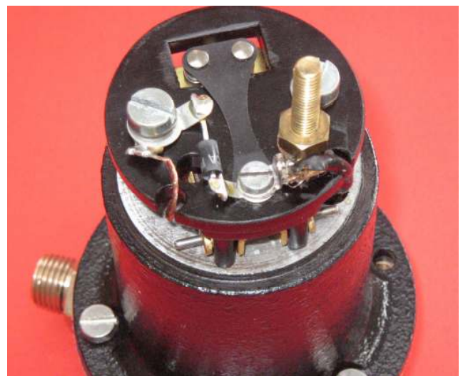
A transil fitted to protect the points
