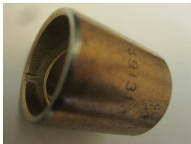
Bi-metal 'wrapped' king pin bush showing the spur groove that feeds the thrust washer.
