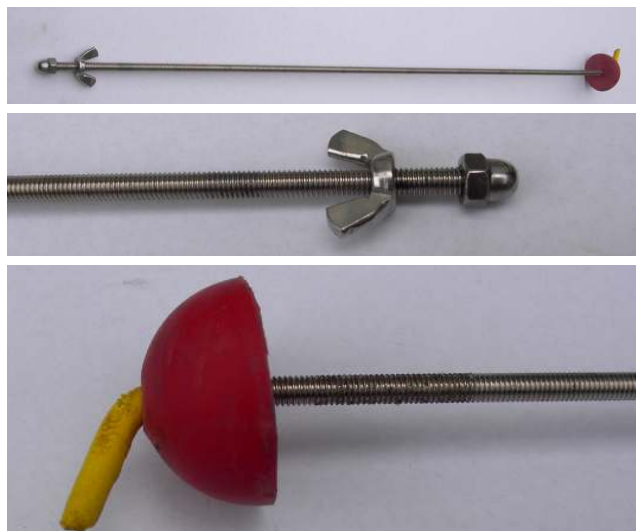
The first three photos show the bonnet support and the detail at each end.
