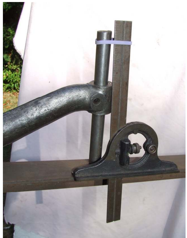
Photo 3 - checking the kingpin inclination angle with a protractor; this can also be used to check the castor angle
