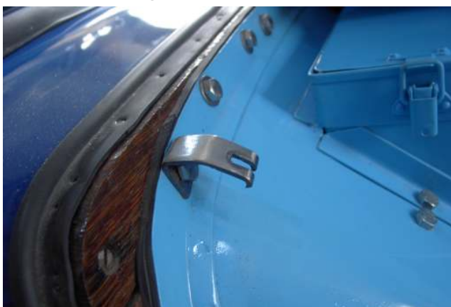
Photos 4 & 5 showing bracket on bulkhead and method of fixing.
