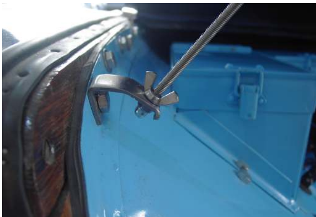
Photos 4 & 5 showing bracket on bulkhead and method of fixing.
