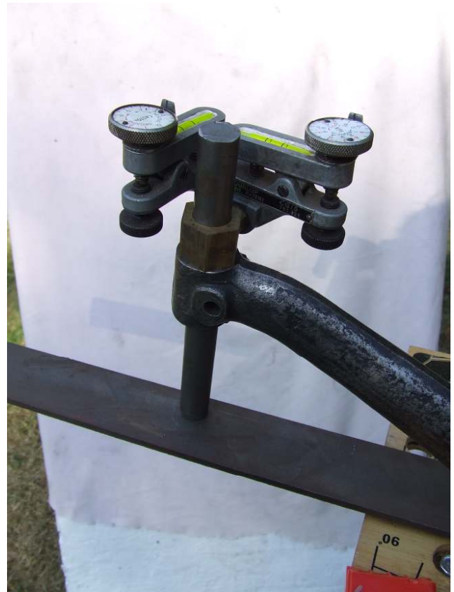
Photo 2 – checking the castor angle with a special Dunlop gauge; this can also be used to check the kingpin inclination angle
