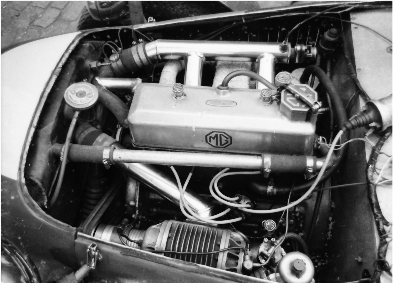
All basic XPAG with long route for the inlet pipe from supercharger to manifold
