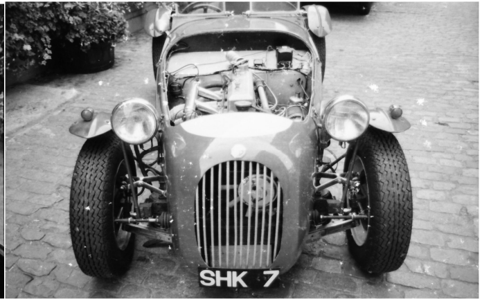
Head on view shows narrowness of design & cooling fan
