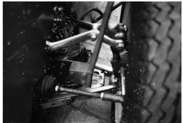
Traditional TD/Y suspension with adaptations and mounting plate for anti-roll bar.
