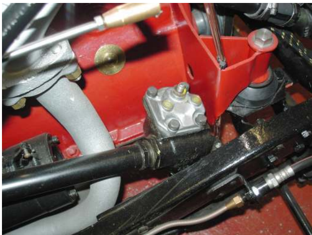
The VW steering box now fitted to Bob Butson's TA. Note also the later type TB/TC front engine mounting.
