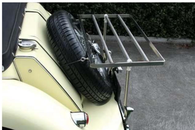
Side view of the completed rack
