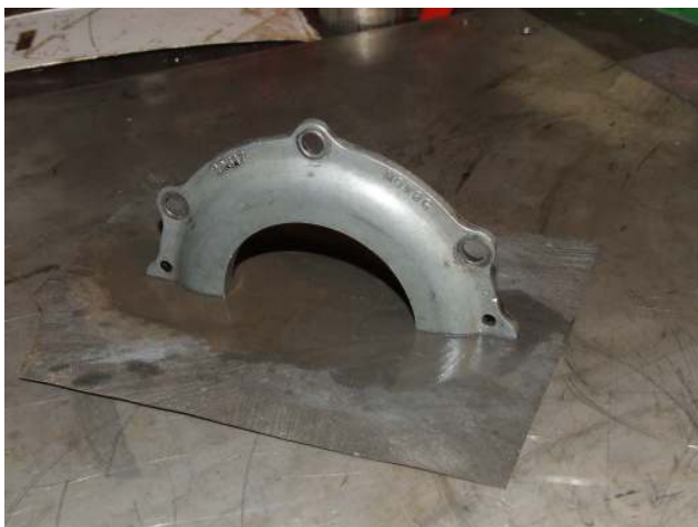
Photo 5 – skimming the cap's flat edge
