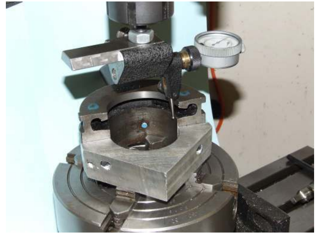
Photo 2- checking the housing with a DTI
