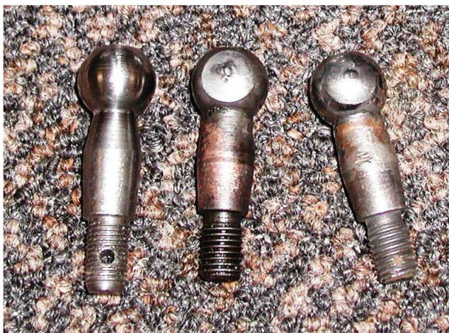
Two examples (on the right) of ball joint wear
