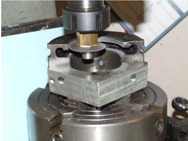
Photo 4 – machining the groove
