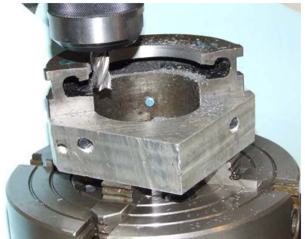
Photo 3 - Machining the housing
