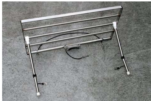
Rack off the car showing method of fixing
