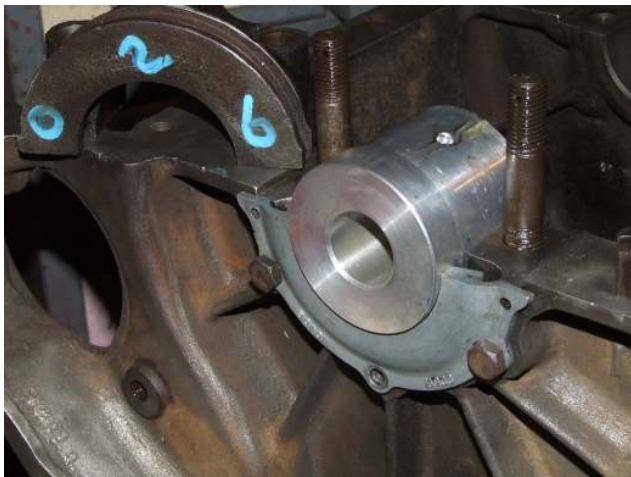
Photo 0 – making up the setting gauge
