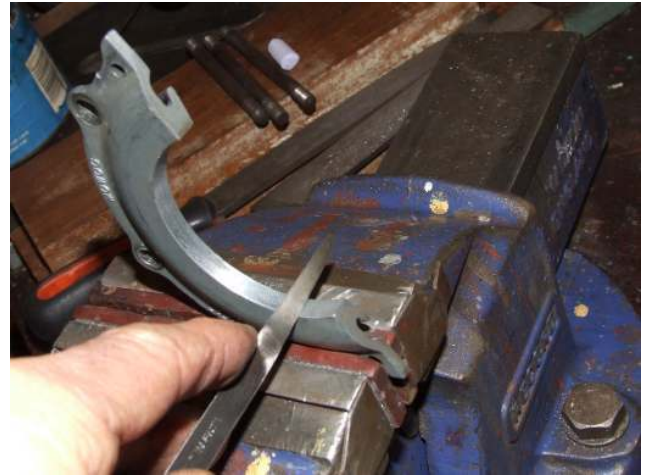
Photo 6 – scraping the cap's surface
