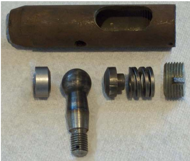
Drag link end assembly
