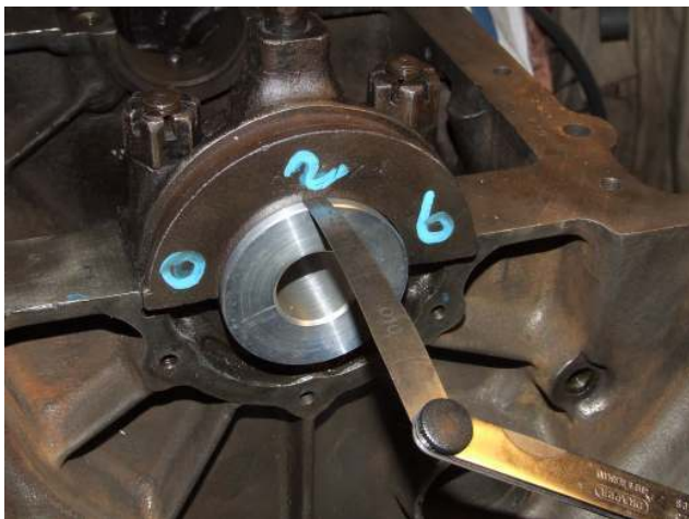
Photo 1 - Feeler gauge inserted between housing and setting gauge
