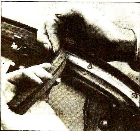
The MGB top rail is held together by these hidden pop-rivets.
