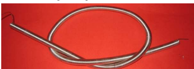
Fig. 4 A Length of Armour Coil Ready To Be Trimmed To Length
