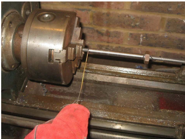
Fig. 3 Winding the Armour Coils
