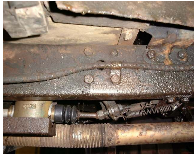
Fig. 1 An original brake pipe and armour coil on 'The Vicar's Car', (complete with 60+ years of accumulated dirt, oil and no doubt some corrosion too).
