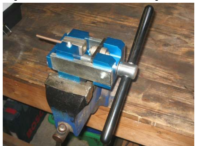
Fig. 6 The Automec Flaring Tool suitable for both 4.8 and 6.35mm tube.
