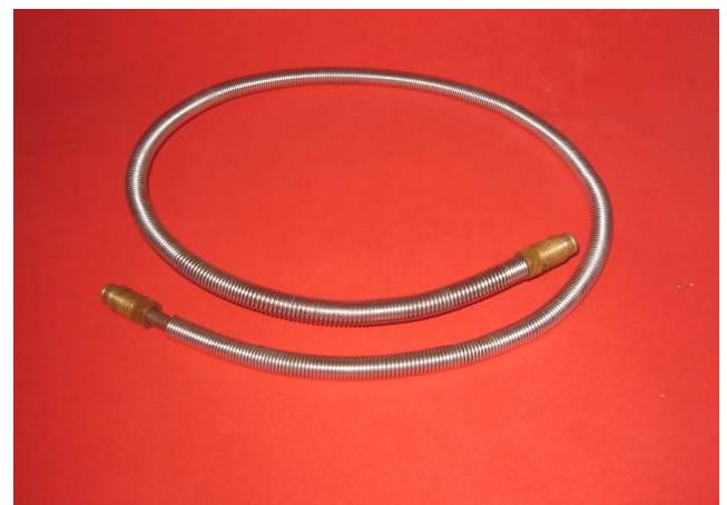
Fig. 7 A finished pipe complete with armour and nipples.
