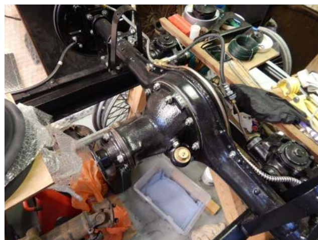
Rebuilt rear axle with 37:8 (4.625) ratio diff obtained from Roger Furneaux.
