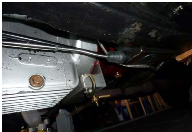
Above: Gaiter and mount fitted to Declan's TD. Below: Seal and cover.
