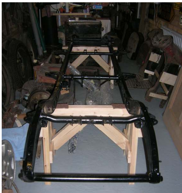
TC0894's chassis after straightening, repair and painting
