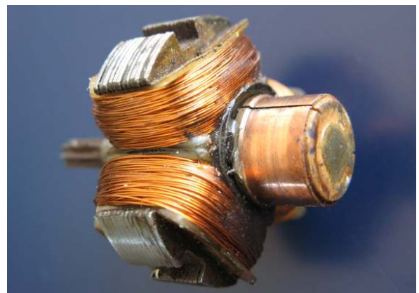
Photo 3 – the armature, having been extracted away from the (front) gearbox and field coil assembly.
