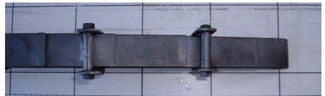
Photo 1 – an after market PA/PB spring with its leaves chopped off square.
