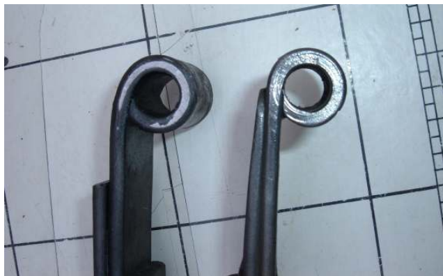
Photo 3 – comparison of ‘eyes’ at the front of the spring; the spring on the left is an after-market PA/PB front spring; the one on the right is an original TC front spring. Although perhaps difficult to spot, the ‘eye’ of the spring on the left is slightly out of round, whereas the one on the right is perfectly round.
