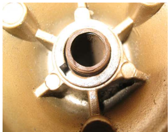
Photo 1 - At the top of the exposed upper end of the column is the bush (Felt) that wraps around the shaft inside the column itself.
