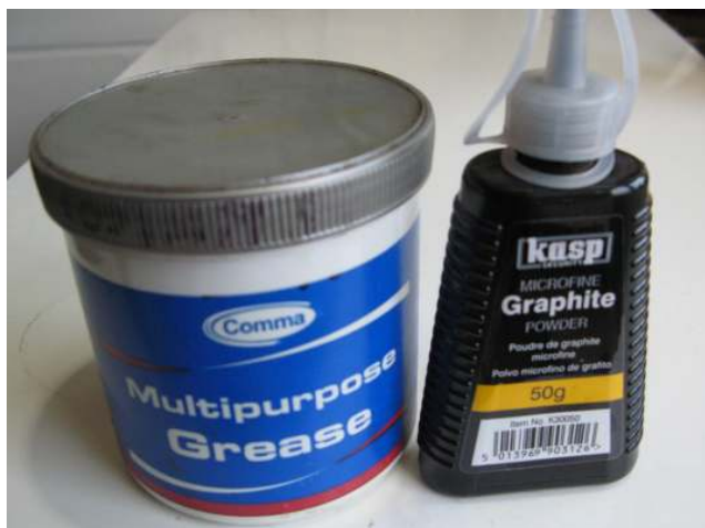
Photo 3 - The Workshop Manuals say that the inner face of the felt should be coated in Graphite Grease to provide the necessary lubrication between column and shaft.
