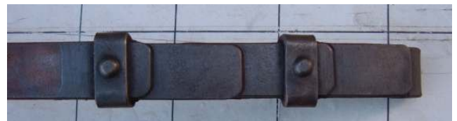
Photo 2 – an original TC front spring with its leaves tapered and chamfered.
