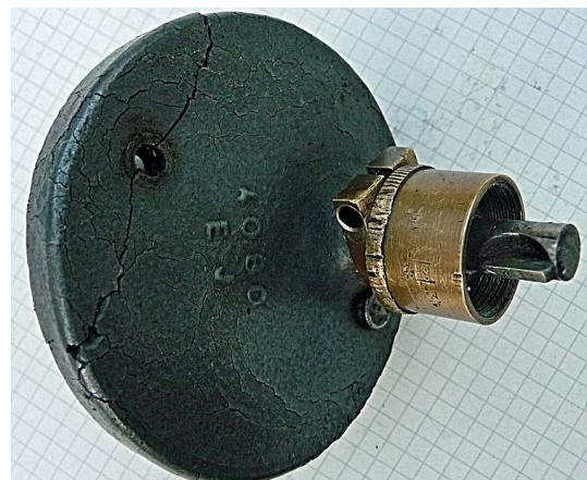
"Before" - with badly cracked casing
