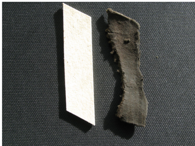
Photo 2 - The New and Old felt bushes show why replacement was necessary!
