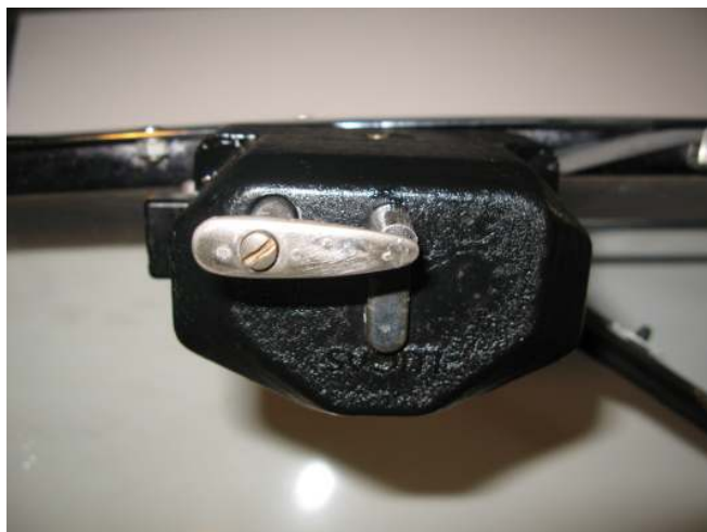
Photo 1 - The familiar view of the Lucas CWX windscreen wiper motor as seen by the passenger!
