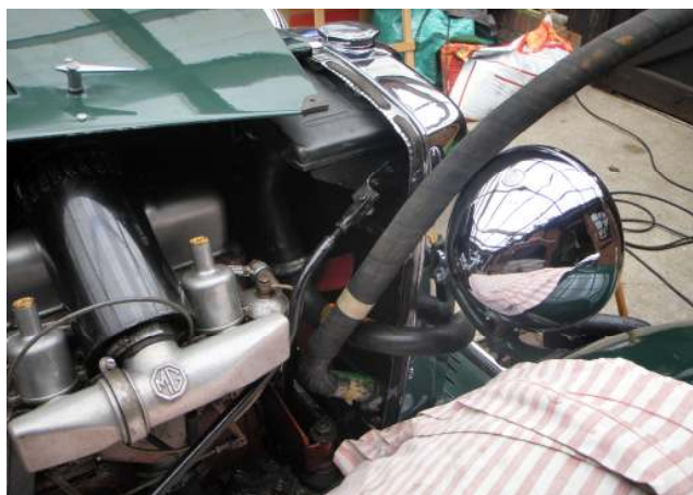
Photo 2 – cleaning the radiator in situ.
