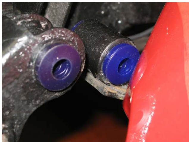
Photo 3 showing the new polyurethane bushes now fitted.
