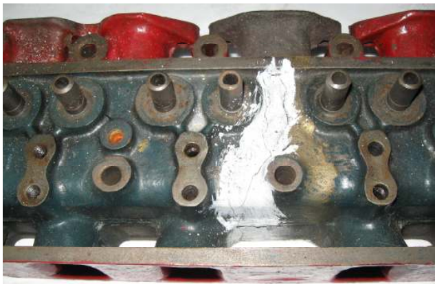
Photo 1 showing the crack – the second time this particular head had developed a crack.
