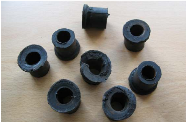
Photo 1- The old rubber bushes removed from the author's TD showing their (considerable) signs of wear.
