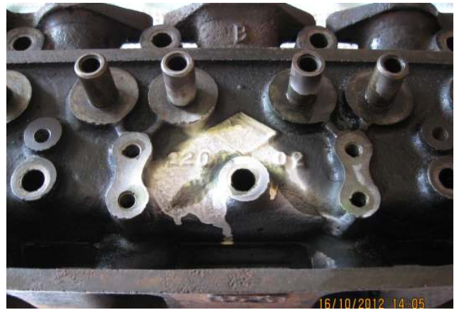
Photo 2 shows the crack in one of Brian's spare cylinder heads
