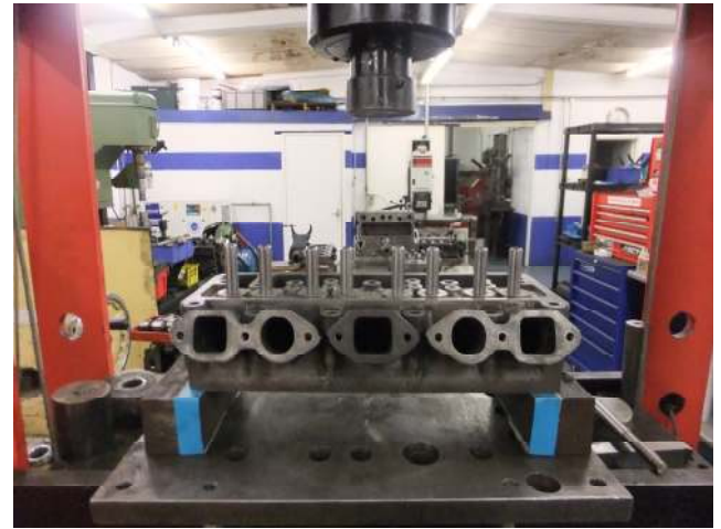
Photo 5 shows the new set of standard valve guides ready to be hydraulically pressed in.
