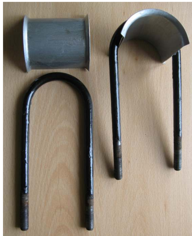
Photo 4 showing the wrap around metal plate which helps prevent axle tube/U-bolt wear.
