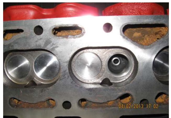
Photo 6 shows skimmed and pressure tested (for the third time!) head
