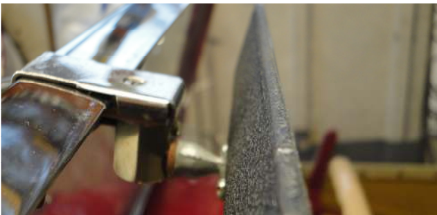
Photos 3 & 4 – showing wide rear view mirror affixed to top rail and stainless steel bracket.
