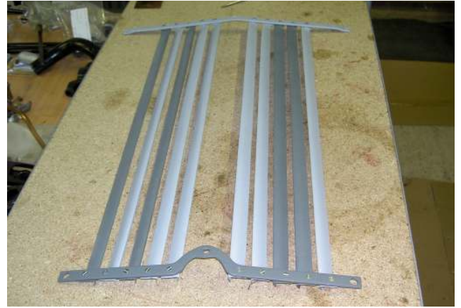
Photos 2 & 3 showing slats attached to bottom rail (above) and front view of top and bottom slats attached to rail (below).
