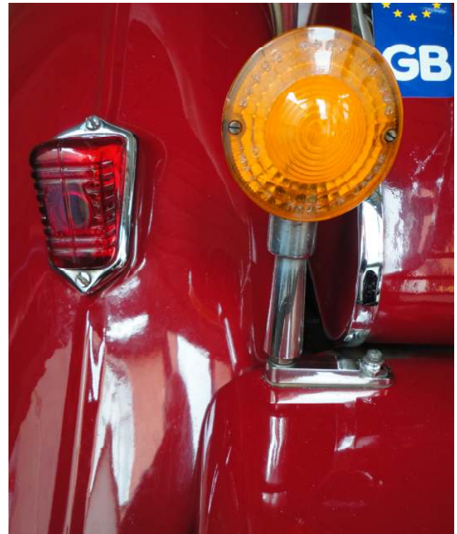
Photo 1 – showing fixing of pedestal type winker light to the rear valance.
