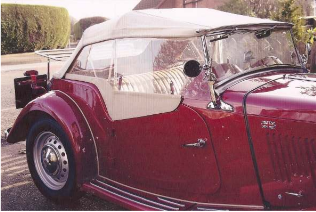
Photo 2 – showing Alan’s polycarbonate sheet side screens (these were featured in Issue 5).
