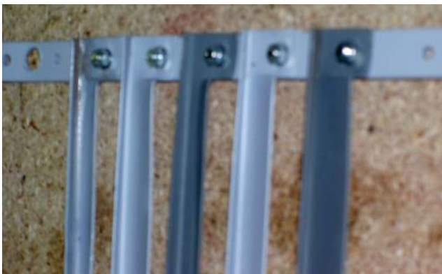
Photo 1 – slats attached to top cross bar
