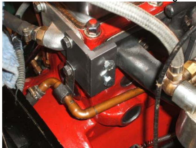
Two more photos from Dieter to show the brackets which prevent the basis plate of the extractor exhaust manifold from distorting.
