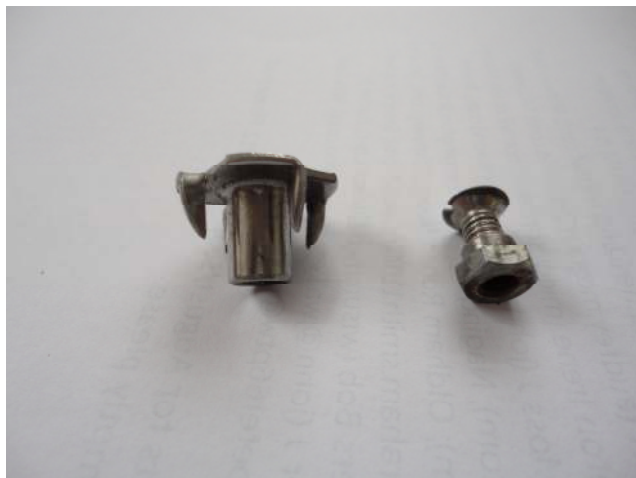
Photo 14 – bonnet fixtures rear and front
