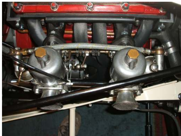
Two more photos from Dieter to show the brackets which prevent the basis plate of the extractor exhaust manifold from distorting.
