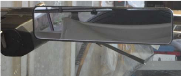
Photos 3 & 4 – showing wide rear view mirror affixed to top rail and stainless steel bracket.
